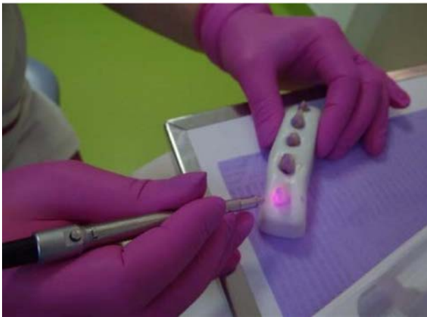
FIGURE 2. The bleaching procedure carried out on each sample with the Epic Biolase USA diode laser 940 nm
