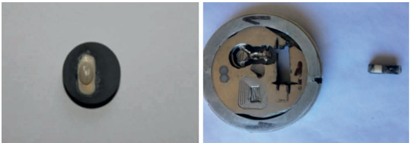
FIGURE 1. Appearance of samples after deposition of ceramics (Noritake T22) on the metal substructure of: (a). TiGrd4; Ti6Al4V, Ti10Zr; (b). TiZrNbTa (sample Ti1)
