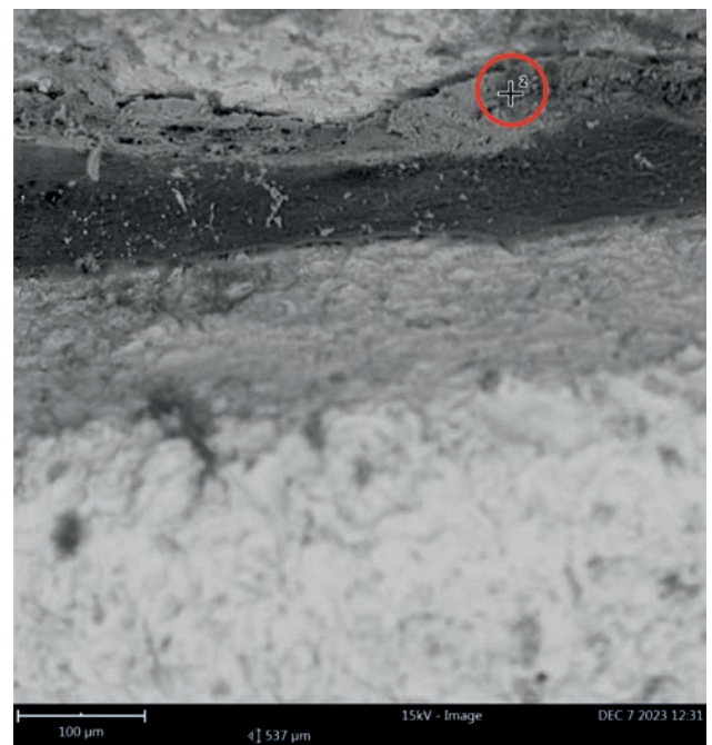
FIGURE 1. Scanning electron microscopy image of sample 6 (coronal region of the implant)
