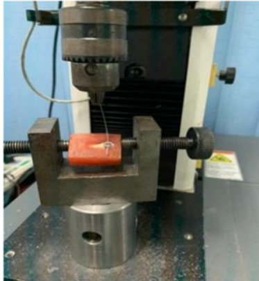
2 Figure 2: Test setup with acrylic block model in Instron Universal Testing Machine.
