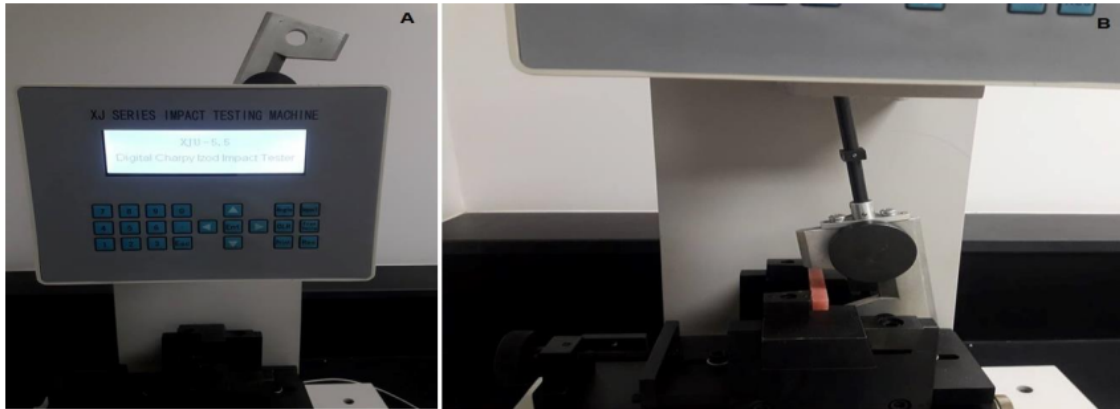
Figure 2 A, B. Charpy's impact testing machine with loaded specimen.
